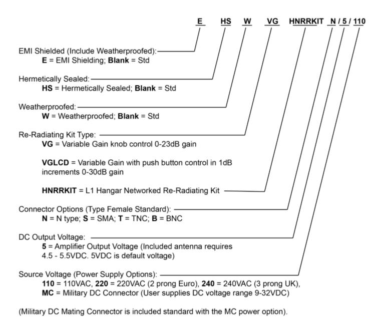
When no external power supply option (AC or DC) is selected, Output 1/J1 is Pass DC Standard.
