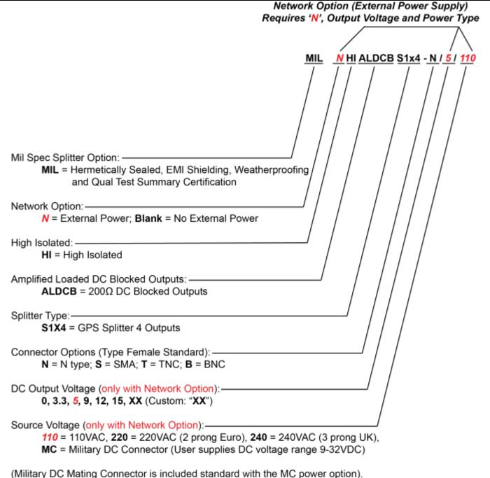
When no external power supply option (AC or DC) is selected, Output 1/J1 is Pass DC Standard. When external power supply option is selected, all outputs are DC blocked standard.
